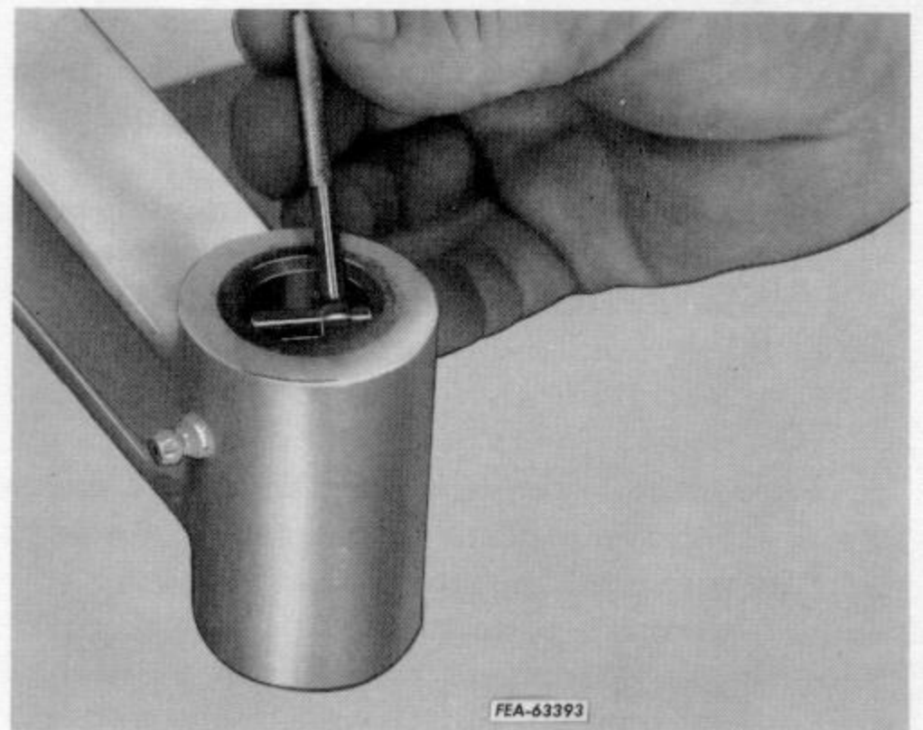
Illust. 10. Checking wear in front axle for steering knuckle pins.
