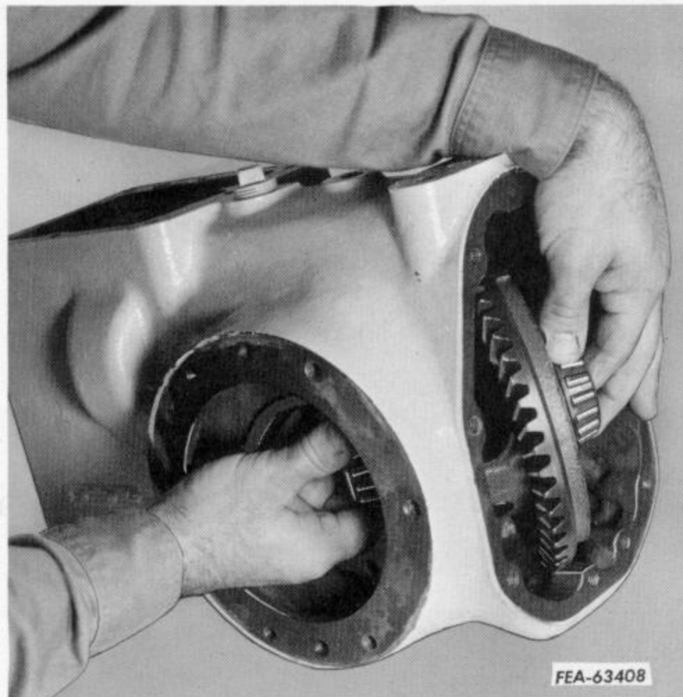
Illust. 26. Removing differential from the transmission case.
